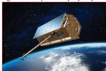
▲ Fig. 3 The PAZ satellite uses SAR to collect images day and night for both military and civilian applications.
