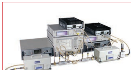
▲ Fig. 2 An MPA-series amplifier used in a vector-receiver load-pull system.
